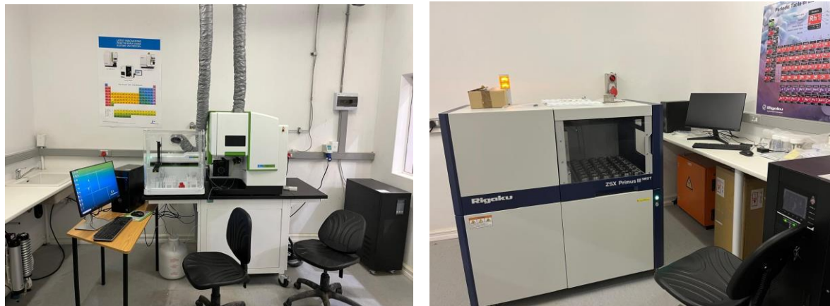
Figure 4: Demo Plant Render Onsite Independent Lab – ICP-OES and XRF Instruments
